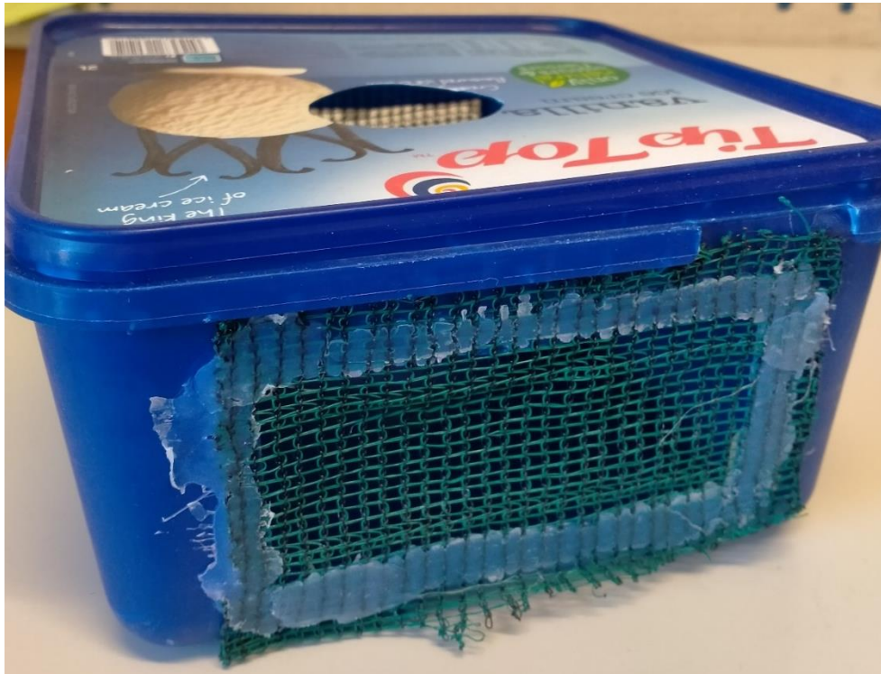
Figure 3.1: Example container used to enclose whelks. Dimensions: 97 x 97 x 80 mm (2 litres) with side panels (approx. 95 x 50 mm) covered with 3mm mesh. Lid has ~45 mm diameter hole, usually covered in 3mm mesh (absent in photo).
