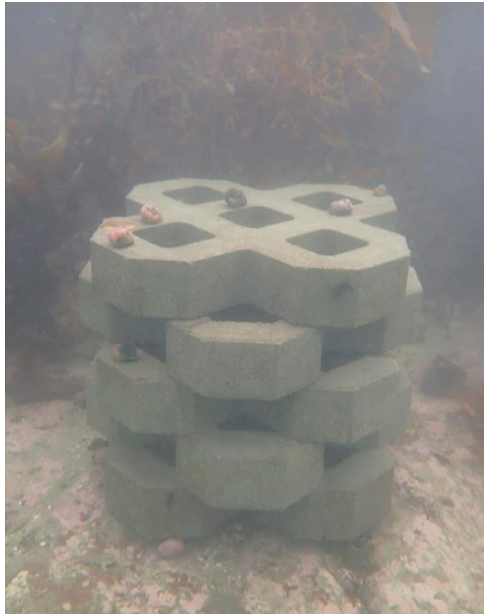
Figure 3.2. Final set up of an artificial reef ‘unit’ in this study. This reef unit is located on the reef edge with no additional structure added.
